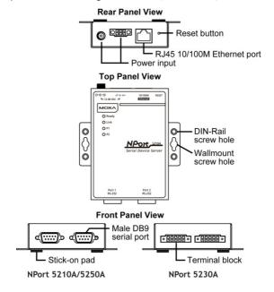
Reset Button—<u>Press and hold the Reset button for 5 seconds to load factory defaults:</u> Use a pointed object, such as a straightened paper clip or toothpick, to depress the reset button. This will cause the Ready LED to blink on and off. The factory defaults will be loaded once the Ready LED stops blinking (after about 5 seconds). At this point, release the reset button.
