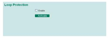
Check the Enable box and click Activate to enable the Loop protection.
