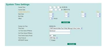
The Moxa switch has a time calibration function based on information from an NTP server or user specified time and date. Functions such as automatic warning emails can therefore include time and date stamp.
