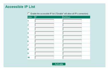
You may add or remove IP addresses to limit access to the Moxa switch. When the accessible IP list is enabled, only addresses on the list will be allowed access to the Moxa switch. Each IP address and netmask entry can be tailored for different situations:
