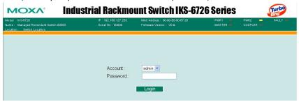
**NOTE** By default, no password is assigned to the Moxa switch's web, serial, and Telnet consoles.
